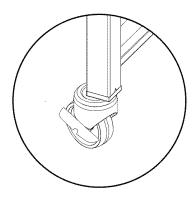
Insert caster into holes on <u>outside</u> corner of caster plug as shown.
